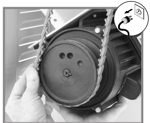
Figure 11. Installing the belt guard.
